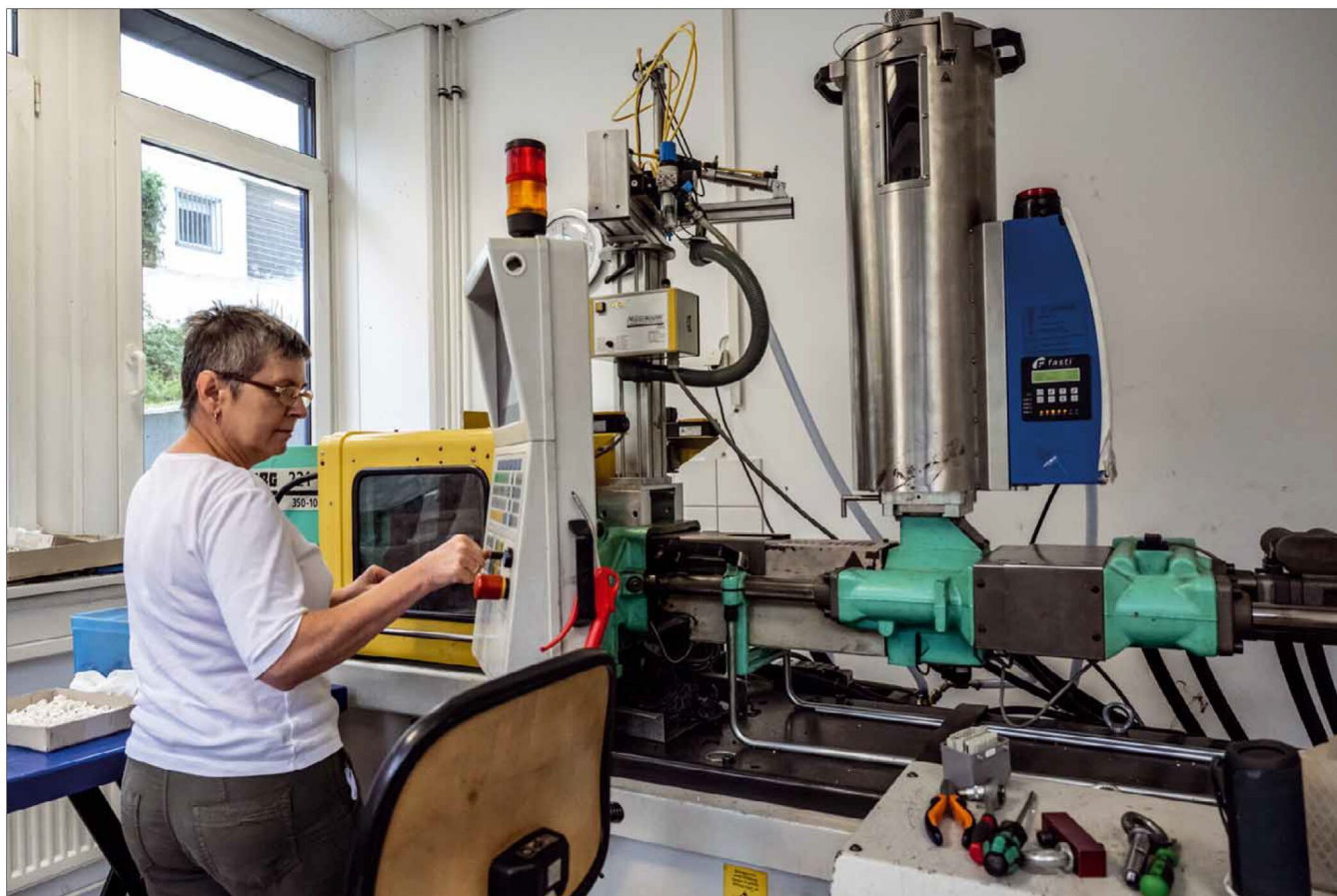
Overmolding metal parts with plastic is a process that WBT has perfected over the years
