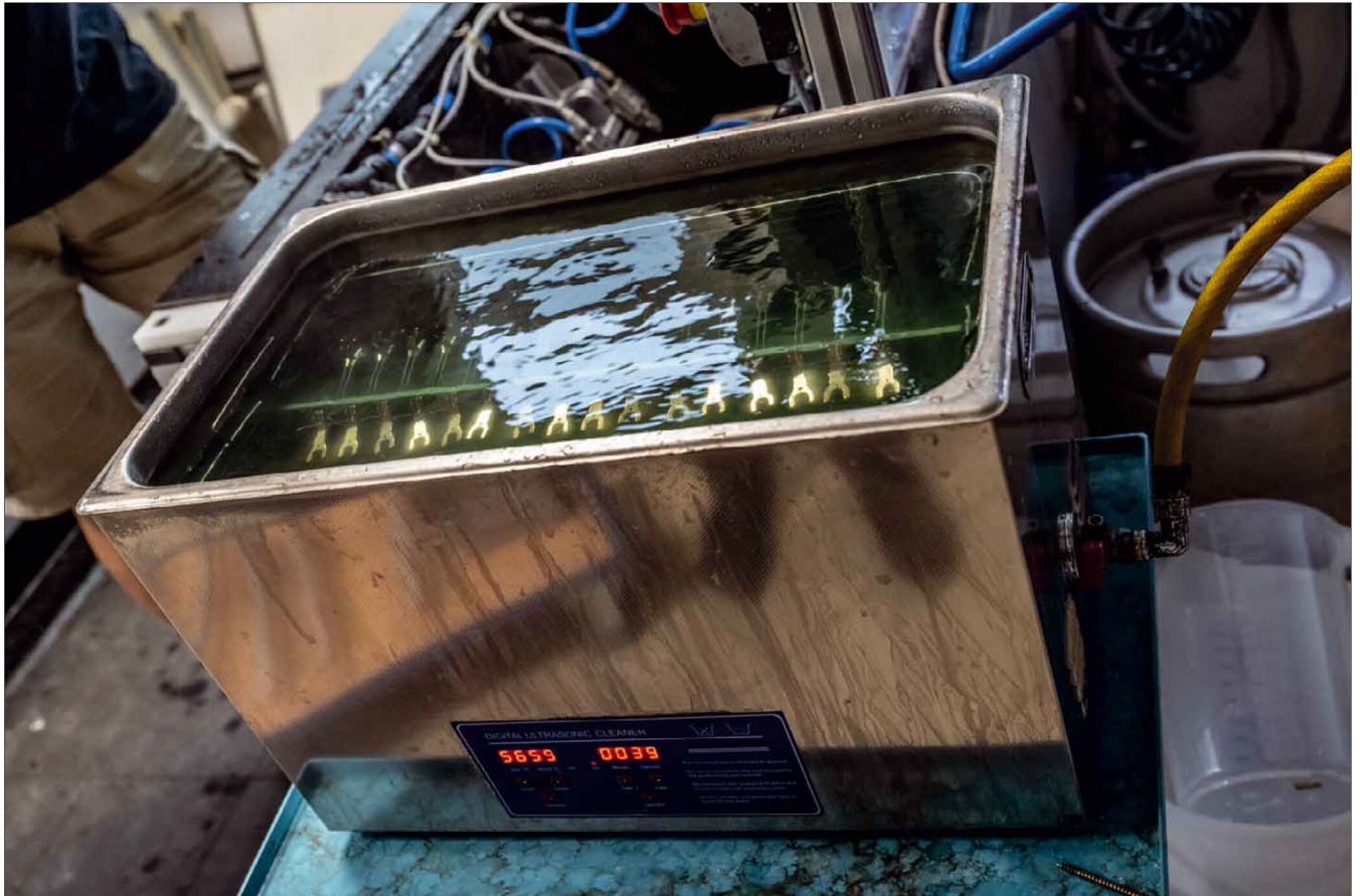
The cleaning procedure for the contact elements also includes a pass in the ultrasonic bath
